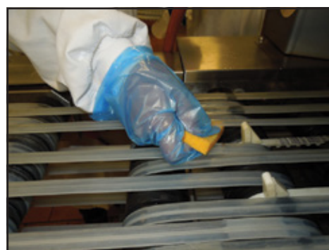
Zone 1 and Zone 2 testing should include swabs taken after equipment has been turned on and gear boxes and belts moving to release hidden biofilms in hard to clean components.
